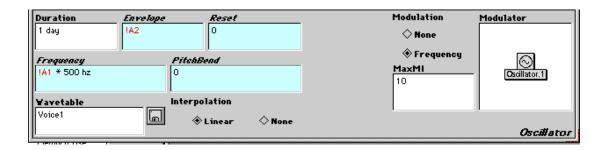
The oscillator prototype includes a modulator, which is also an oscillator. Users may replace this oscillator with another oscillator or sound source by dragging the new input into the Modulator window. An example of a parameter field for a modulator is shown below.
