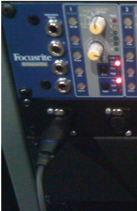
4. The jack shown above is hardwired to channel 1 of the Focusrite pre-amp unit. The individual pre-amp is shown below:
