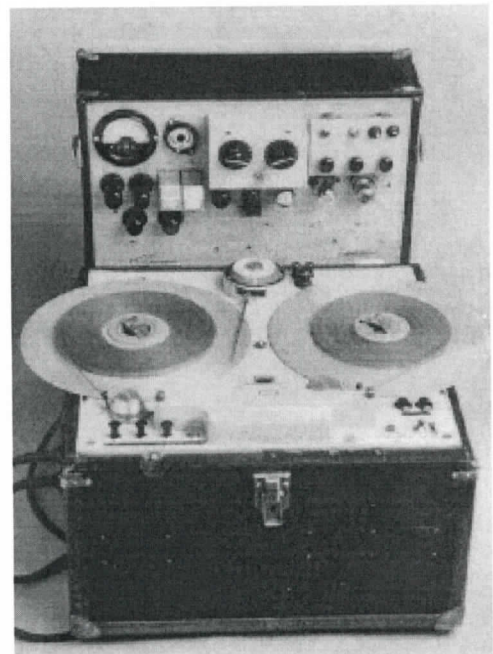
Fig. 64. AEG magnetic tape recorder, ca. 1935.
