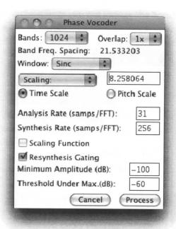
Adjusting the time scale will time-stretch a sound and pitch scale will generally shorten a sound raise the pitch.
