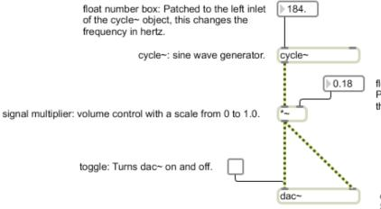
float number box: increments in decimal places. Patched to the right inlet of the signal multiplier, this changes the loudness.
