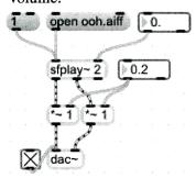
j. To change the volume of the two channels independently, simply create another float box. Attach the left outlet of one float box to the right inlet of one [\*~]. In the patch shown below, the left channel will playback at 20% original volume, while the right channel will playback at 90%.
