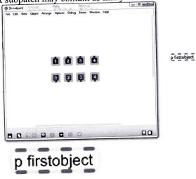
\*It is important to note that the order of the inlets/outlets does matter. If you have set up connections and decide to change the order, re-check to make sure that the cables correspond!\*
