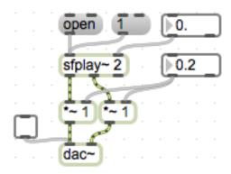
j. To change the volume of the two channels independently, simply create another flonum. Attach the left outlet of one flomun to the right inlet of one [\*~]. In the example below, the left channel will playback at 20% original volume, while the right channel will playback at 90%.
