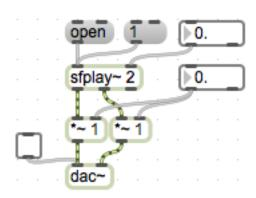
i. We can update the math happening in the [\*~] object by sending new numerical values into the objects' right inlet. The value that is set in the flonum object will be sent to each [\*~] concurrently, changing the volume of each channel by the same amount. So, in the following example, each channel will be heard at 20% of their original volume.
