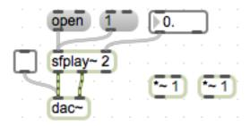
d. Now delete the patch cords connecting [sfplay~] to [dac~] by clicking on each of the cables and pressing the delete key one at a time.
