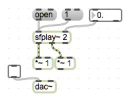
f. Now connect the outlet of the left [\*~] to the left inlet of the [dac~], and right to right.
