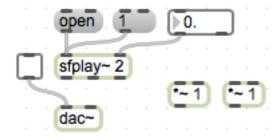
e. Click and drag the [dac~] and the toggle to make room for our two new [\*~] objects. Connect the channel one outlet of [sfplay~] to the left inlet of one of the [\*~] objects, and the channel two outlet to the other.
